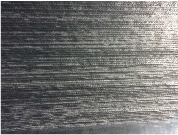
Fig. 4 Example of a Weld Overlay Surface
